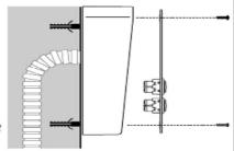
UP11D. Da incasso, ad 1 pulsante / Flush mounting, with 1 push-button / À encastrement, à 1 bouton-poussoir De encaje, con 1 pulsador / De encaixe, com 1 botão / Wandmontage mit 1 Taster
