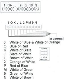
NOTE: There are many different versions of the handsets for STATUS (SML), so a picture of the insides and terminal markings is the best way to get a positive identification.
